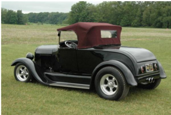
We now own a black 1928 Ford roadster with a cranberry interior and top that I refer to as a Streetrod. The top will drop or come off in a matter of minutes. This car has a Buick 3.8 V6 engine with lots of chrome! It is hooked up to a 350 automatic transmission, and the rear end is a ten bolt with coil-overs. It has a dropped front axle, which puts it right down in the grass.
